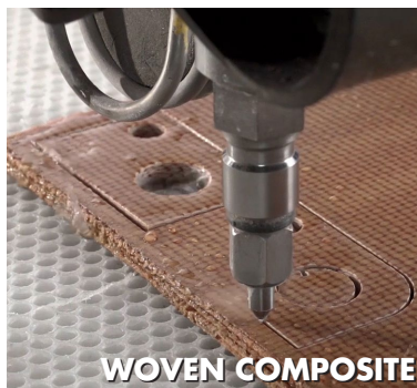
Potential Delamination with Standard Cutting Head: Scrap Part & Restart Production
