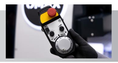
The OptiMAX® Bridge Pendant allows the waterjet operator to move the Cutting Head and the Bridge along X, Z and Y Axis, dial in the cutting head to the work piece or perform dry runs to test drawings or materials.
